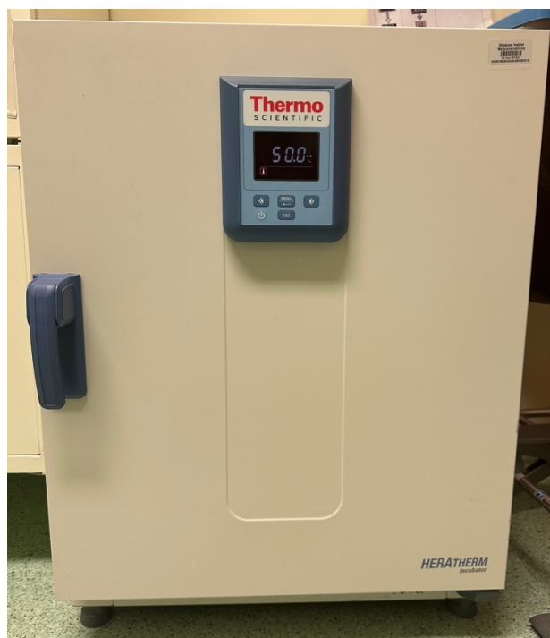
Rycina 3. Ciepłarka laboratoryjna Heratherm Advanced Protocol Security Thermo Scientific, Thermo Fisher Scientific, USA.
