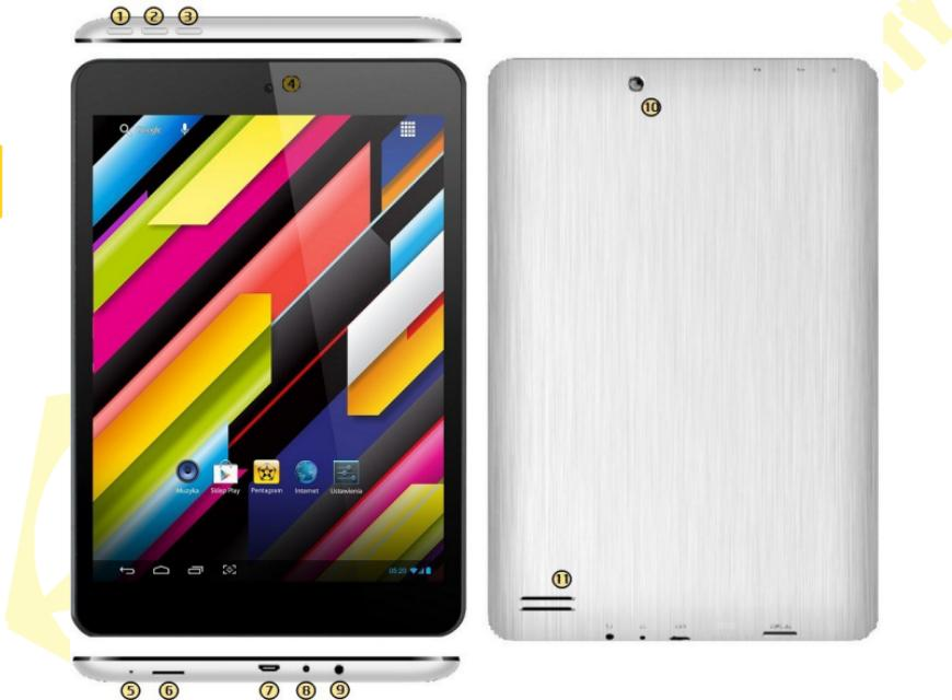
1. Power button - to turn on or off the device, press and hold this button for approx. 4 seconds.
