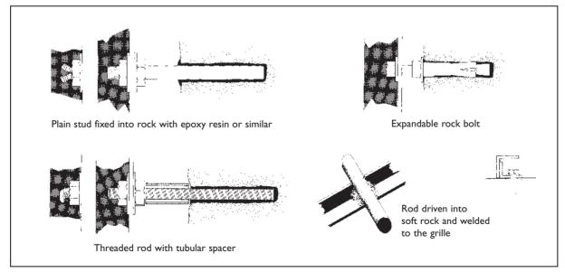
**Figure 11.4** Alternative methods of fixing grilles in position.
