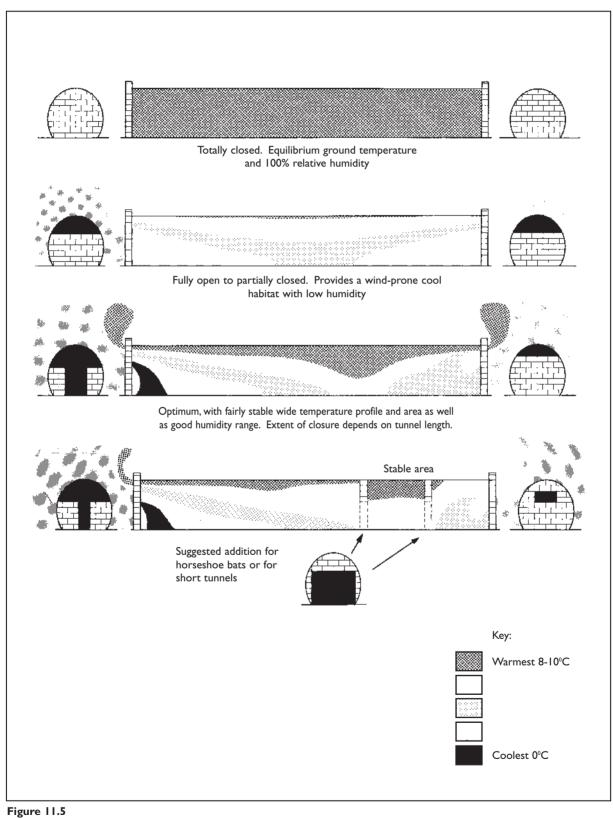
Creating bat hibernacula from tunnels. Air flow, temperature and humidity can be controlled by the design of the end-walls. Winter temperatures and air flows are shown.
