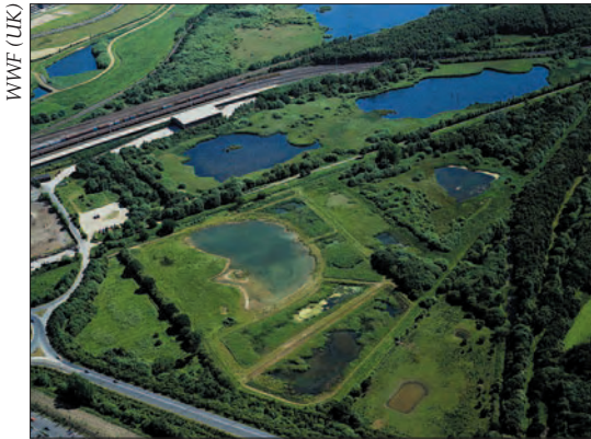
Plate 5.4 The five cells around the semicircular lake in the bottom half of the picture make up a reedbed filtration system, Potteric Carr, Yorkshire, UK.
